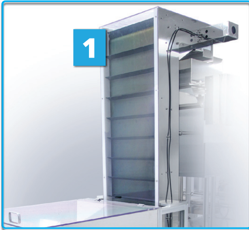
1 Floor Level Bulk Feed Hopper with Cleated Elevator Starts the Process
