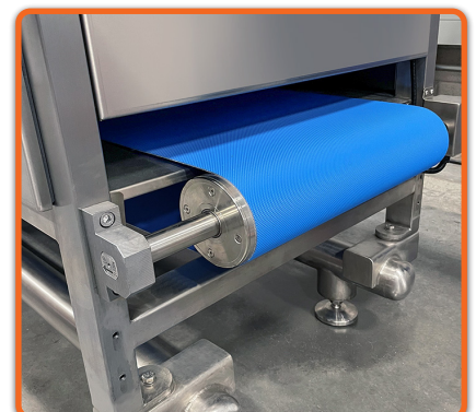
Live-Belt Drive Motor (Inside Roller)
