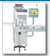
Here the containers enter from the rear. A patented DIVY™ Bottle Handling System senses the bottle density in each lane and directs approaching bottles to the less dense lanes. Bottles continue in lanes under the feed assembly where they are filled by one product drop per lane (1-4 lanes) and exit at the front of the machine.
