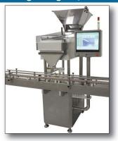
In this photo the bottles enter from the left, are filled from a single drop and exit to the right.
