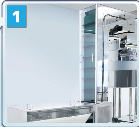
Floor Level Bulk Feed Hopper with Cleated Elevator Starts the Process
