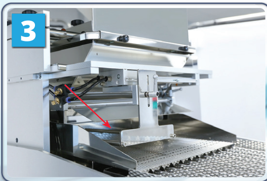
The Adjustable Variable Speed Diverter Bar Above the Product Channels, Sweeps Left & Right to Eliminate "Twinning"
