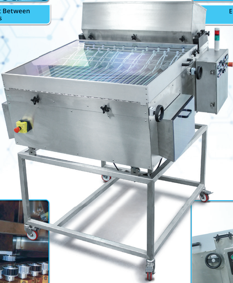
All Rollers Driven By a Single Timing Belt
