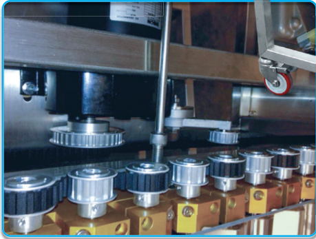
All Rollers Driven By a Single Timing Belt
